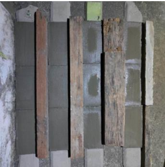
Fig. 4. Curing of Trapezoidal Concrete
