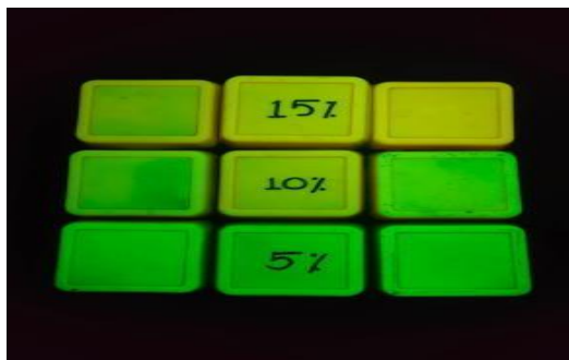
Fig. 11. Glow-in-the-dark concrete topping-based road marking
